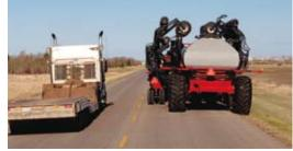
Patented rearward folding toolbar design provides narrow transport for stability and safety, providing operator peace of mind on busy highways. The compact footprint also allows for easy storage inside during the off season.
